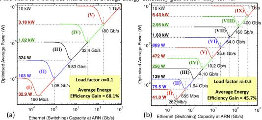
Fig.3. Upgrade trajectories from 1Gb/s $\rightarrow$ 1Tb/s: (a) 5 generations for  $\alpha$ =0.1, efficiency gain  $\eta$ =68.1%; (b) 9 generations for  $\alpha$ =0.3, and  $\eta$ =45.7%.
