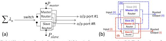
Fig.1. (a) Master-slave configuration for edge-routers; (b) Schematic of two successive generations (I) & (II) of master-slave configurations.
